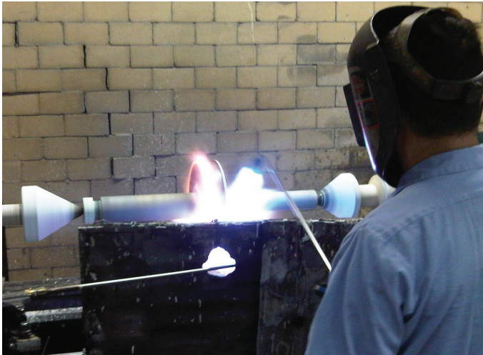
Fusing Colmonoy® 52 M onto Blow Out Preventer Ram
