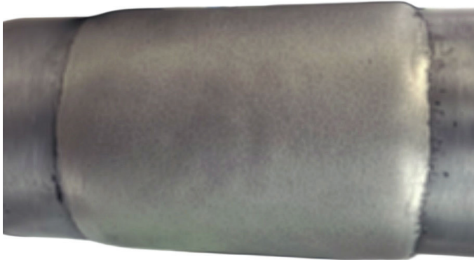
Colferoloy™ 6005 coating applied to an under carriage bushing by the Sprayweld™ process and furnace fused at 1115°C (2040°F).
