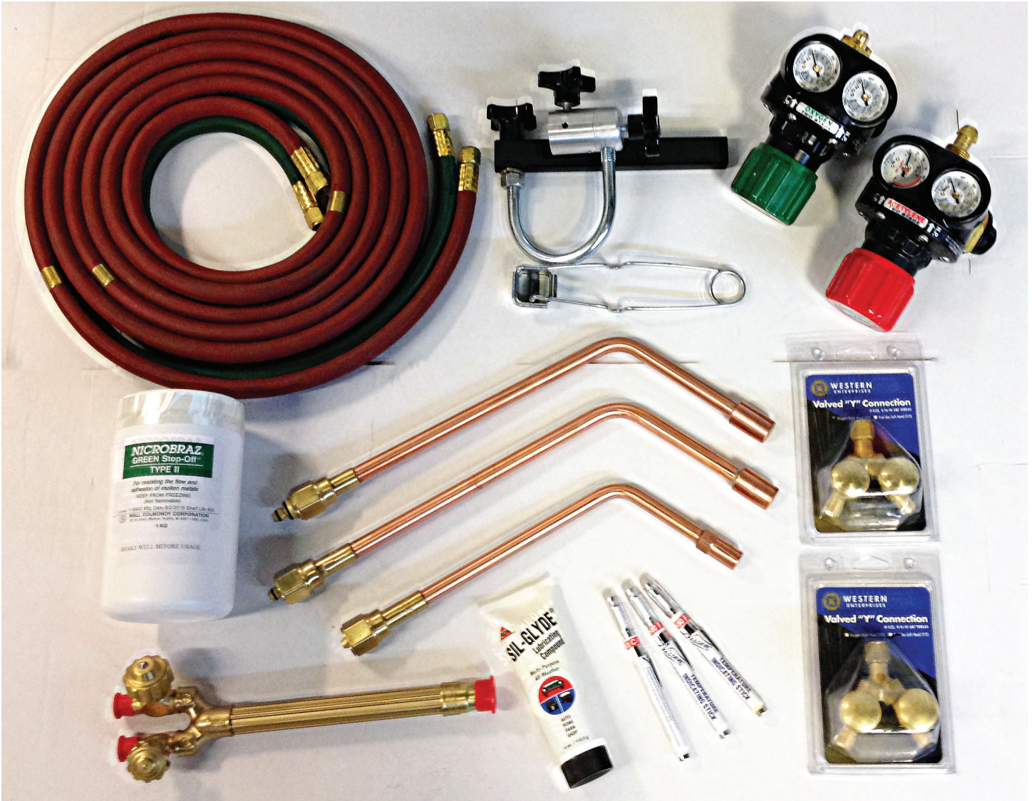
Figure 9-5. The Spraywelder™ Equipment Group includes accessories needed in a Sprayweld™ Process Installation: Two-stage oxygen and acetylene regulators, fuel gas supply hose (15-ft), fusing torch handle (310 H.D.), three complete nozzles (type 11, sizes 8, 12, 15), two Y-connectors, friction lighter, temperature crayons (93, 260, 343°C) (200, 500 & 650°F ), and a pint of Green Stop-Off™ Type II Inhibitor (not shown).
