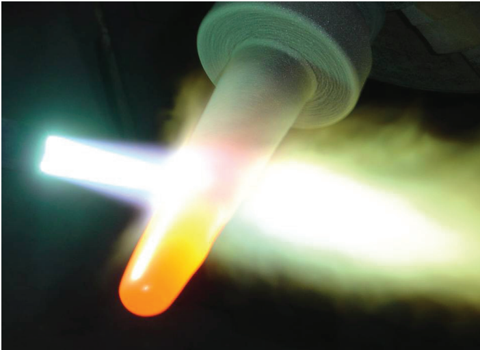
A glass mold plunger coated with Colmonoy® 42 , being torch fused.
