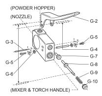
All torch handle assemblies have built-in reverse flow check valves to protect against accidental ignition in oxygen and fuel-gas supply hoses.
