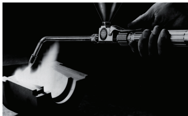
Fusewelder™ Torch spraying Colmonoy® 227 on glass container moulds
